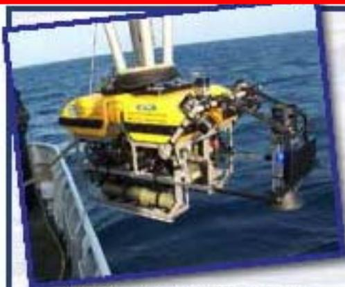
A gas capture device was added to the front of the GOV-Hercules remotely operated vehicle for several dives. Image courtesy of the NOAA Ocean Explorer Program.
